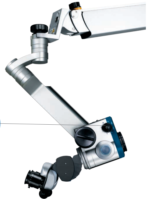
Turning knob for the filter disk
