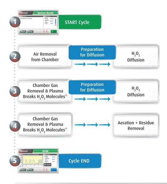
Plasma breaks down Hydrogen Peroxide  $(H_2O_2)$  molecules into Water  $(H_2O)$  and Oxygen  $(O_2)$  outside the chamber
